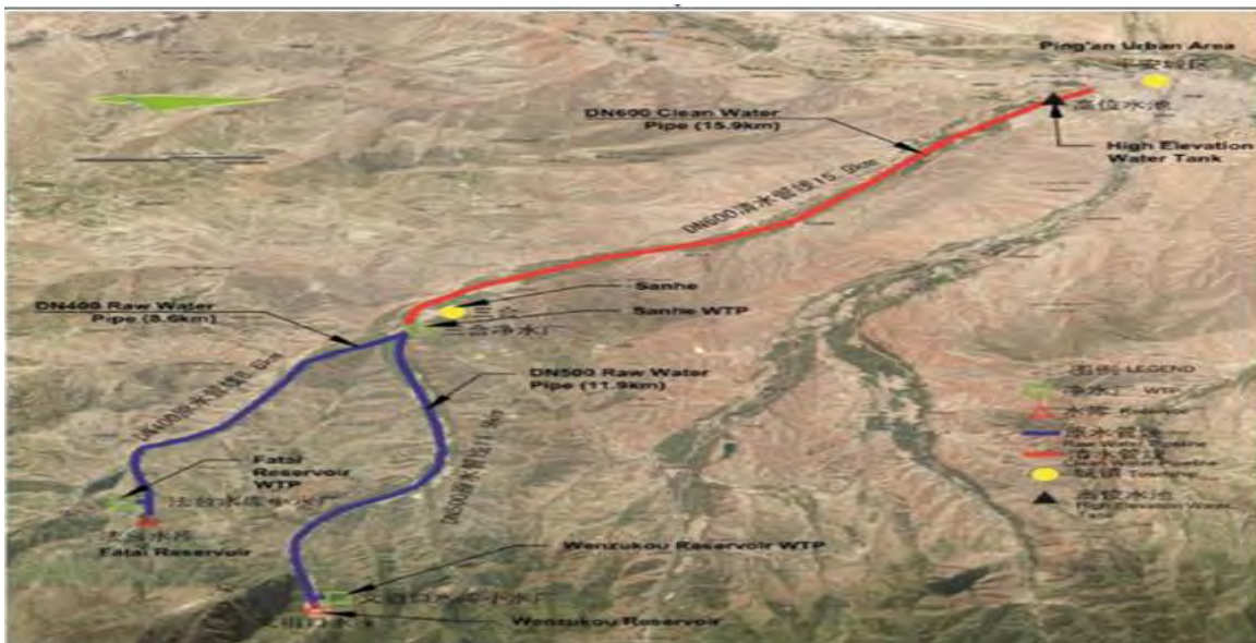
Figure 1-6 Proposed Raw Water and Clean Water Pipe
