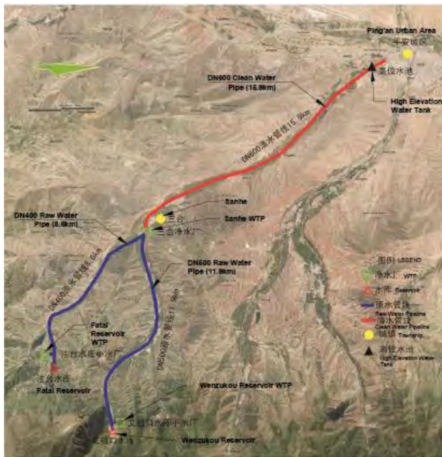
Figure III.15: Scheme of the proposed urban-rural water supply component
