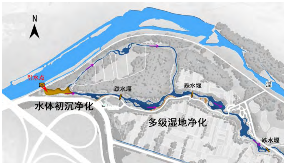
Figure III.10: Huangshui River water intake point for Yizhou Wetland Park
