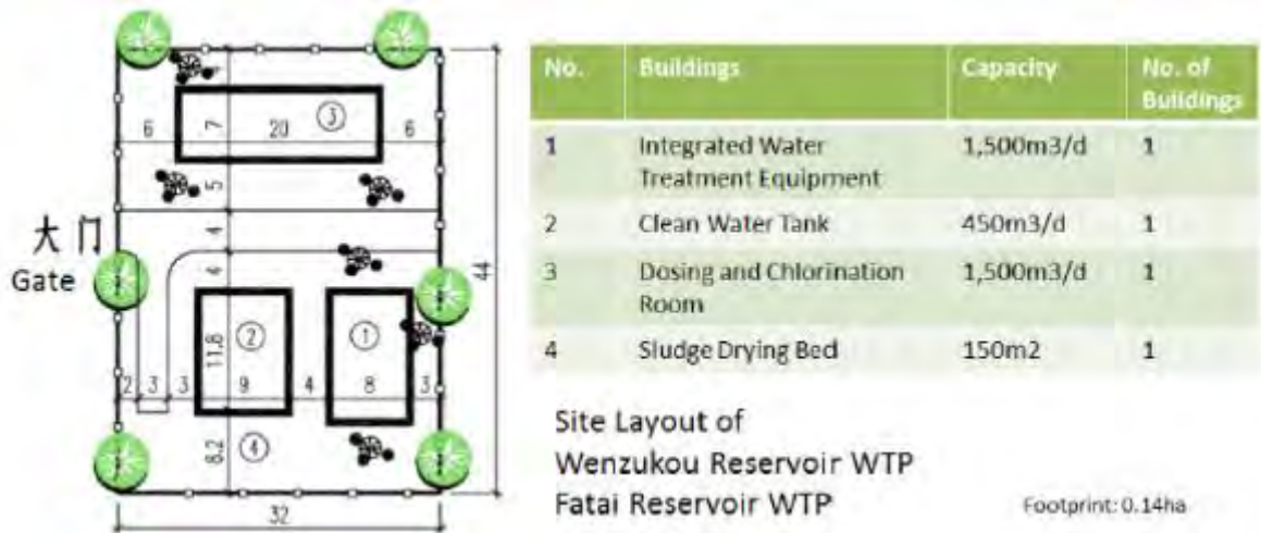
Figure III.19: Wenzukou and Fatai WTP Site Layouts
