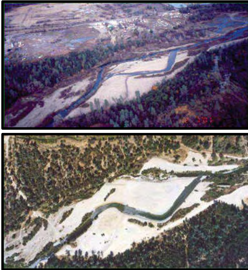
Figure 3-5 Channel changes to increase fish spawning habitat in Clear Creek California. Above = before; Below = after. http://wildfish.montana.edu/Cases . Accessed 27.03.2104
