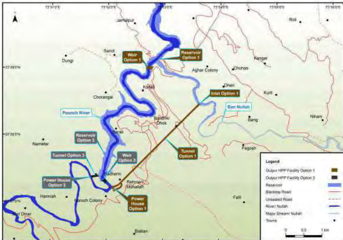
Figure 2: Gulpur Hydropower Project Layout for Option 1 and 3 and Environmental Flow Site Locations
