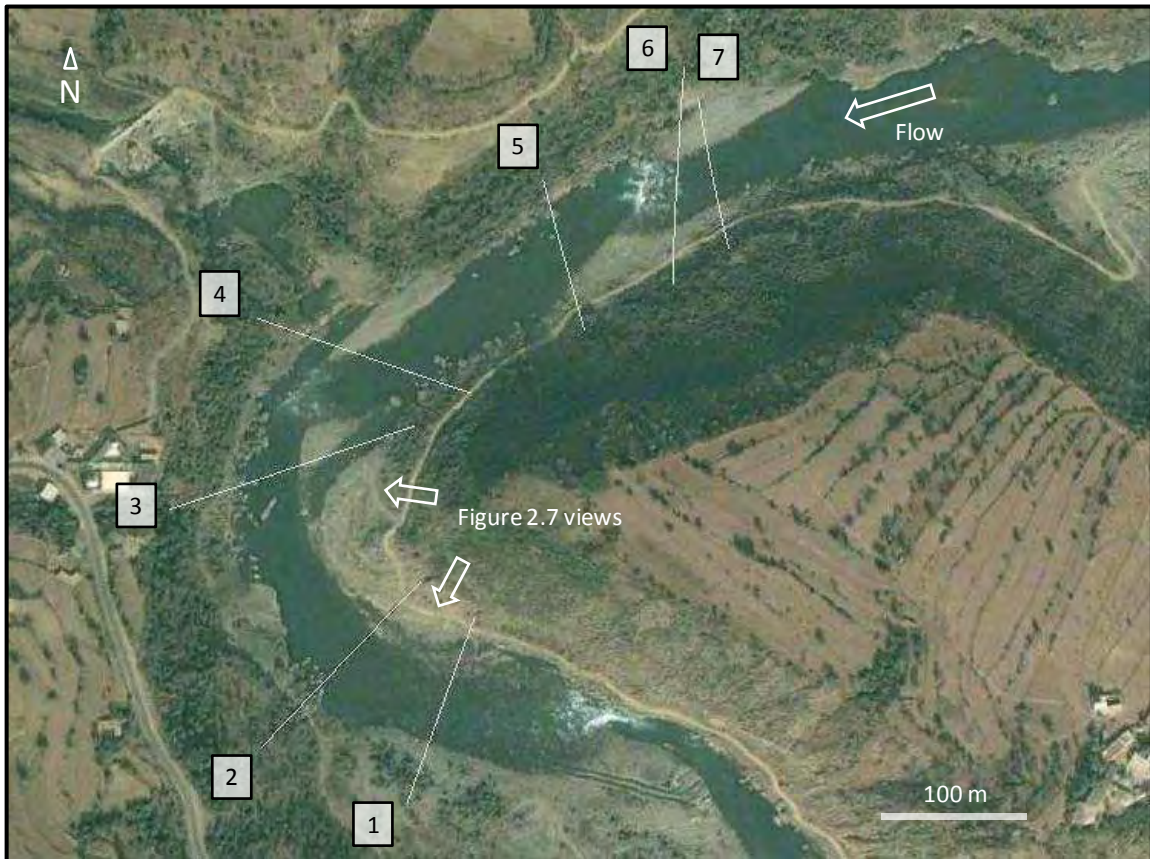
Figure 5-35: The positioning of surveyed cross-sections at EF Site 3 (Gulpur Bridge) using a 1 November 2005 aerial view
