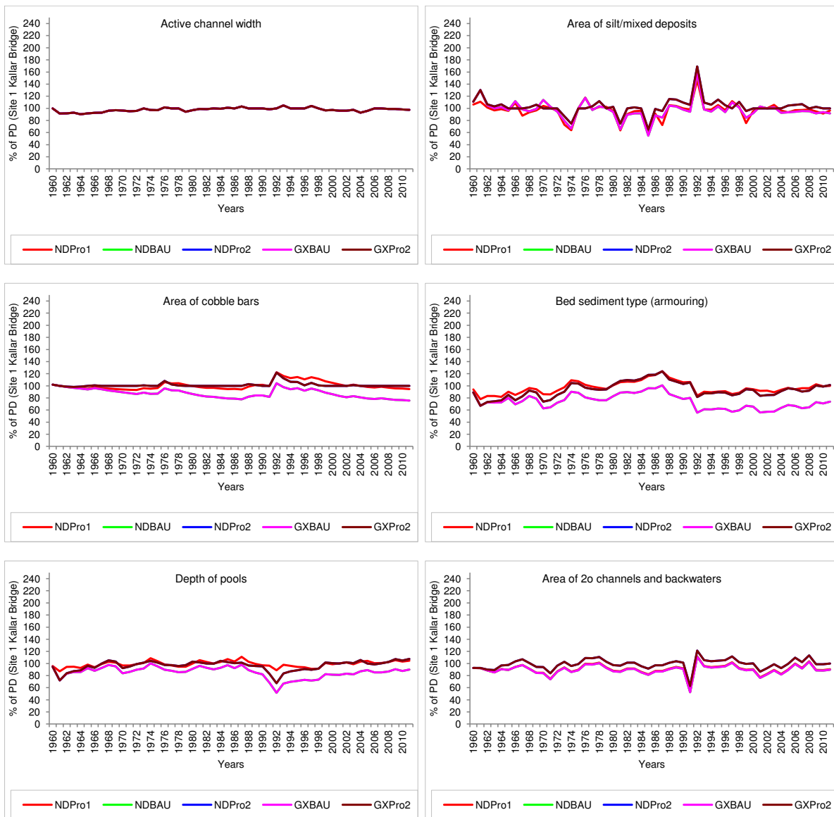
Figure 6.1 Time-series of predicted changes in geomorphological indicators at EF Site 1. Scenario lines not visible are hidden by those showing.
