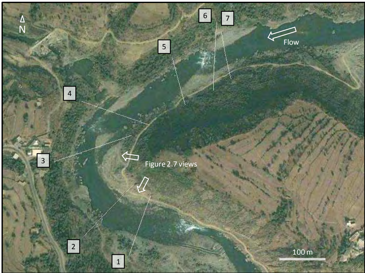
Figure 2.6 The positioning of surveyed cross-sections at EF Site 3 (Gulpur Bridge) using a 1 November 2005 aerial view.
