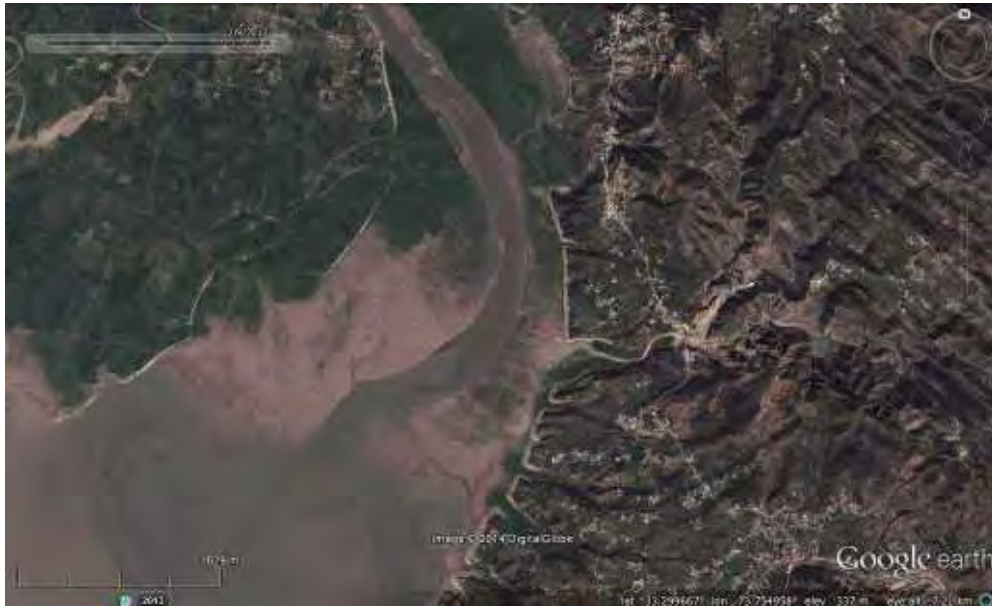
Figure 2-2 Large volumes of sandy sediments deposited where the Poonch River enters Mangla reservoir.
