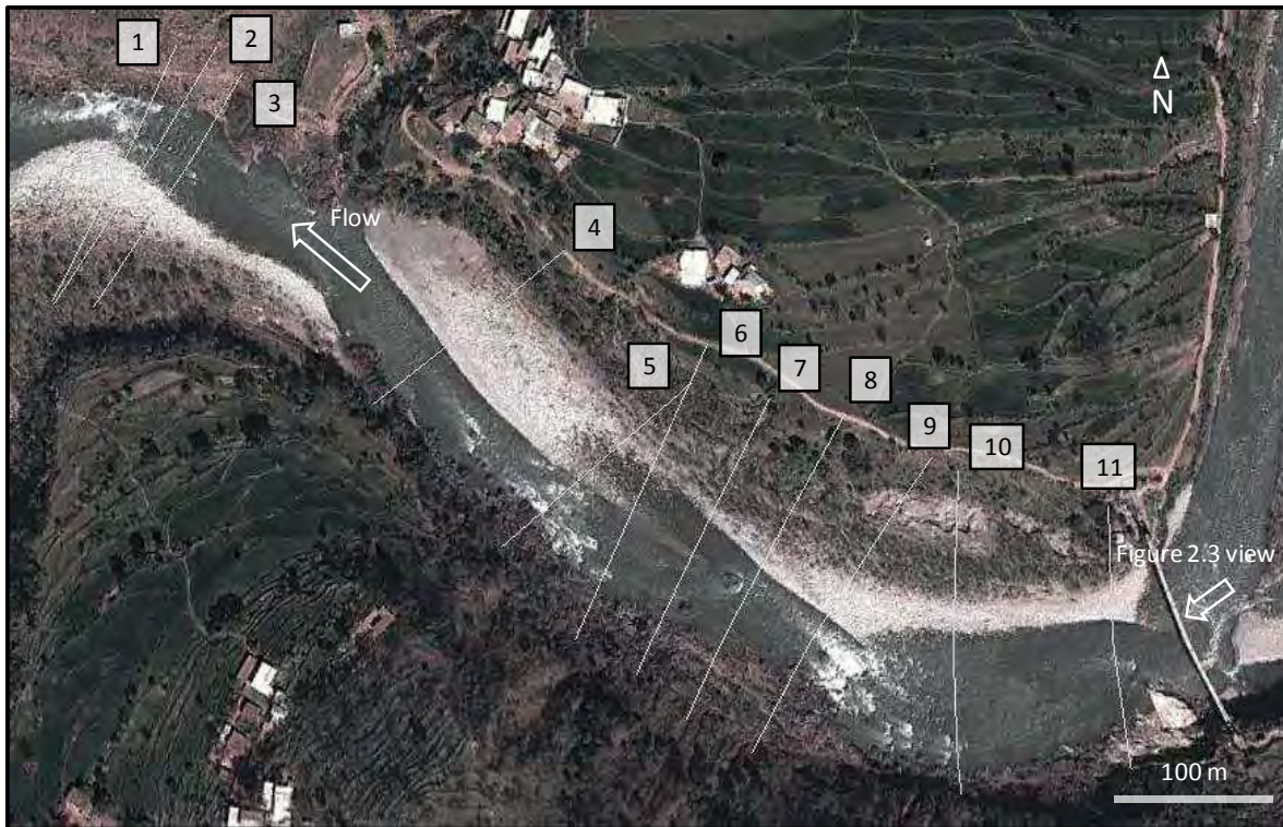
Figure 2.2 The positioning of surveyed cross-sections at EF Site 1 (Kallar Bridge) using a 15 March 2010 aerial view.
