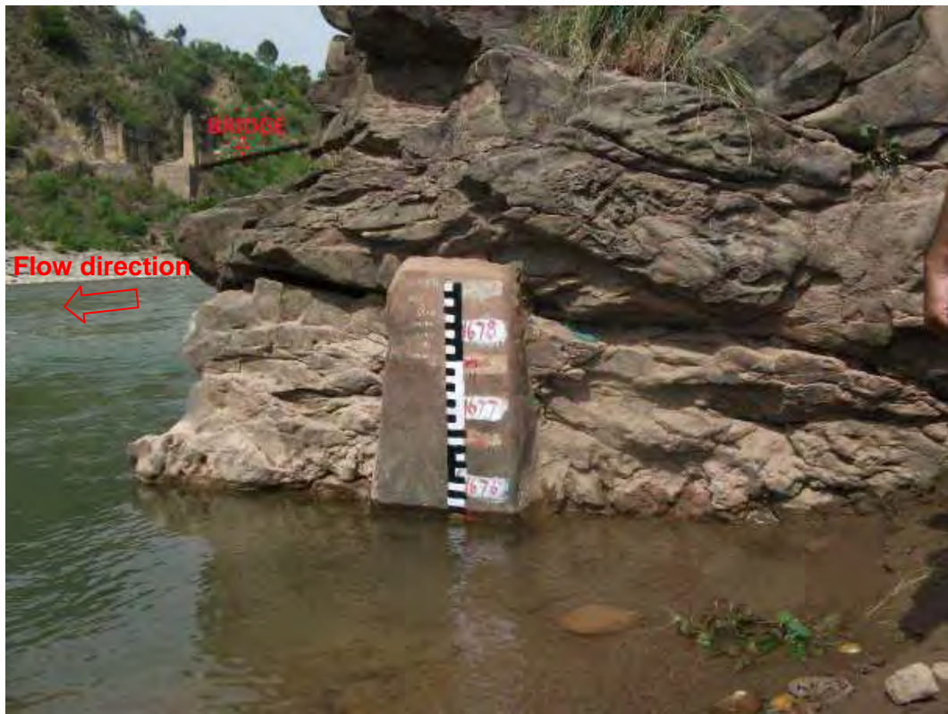
Figure 4: Poonch River at Kotli – Gauge Location is downstream of confluence of Poonch River and Bann Nullah; the painted gauge is on a rock protruding from left bank of Poonch River
