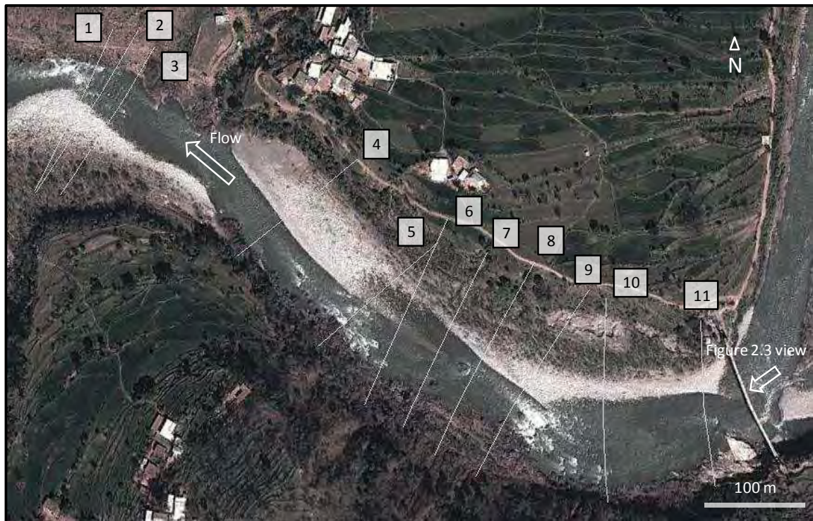
Figure 5-31: The positioning of surveyed cross-sections at EF Site 1 (Kallar Bridge) using a 15 March 2010 aerial view.
