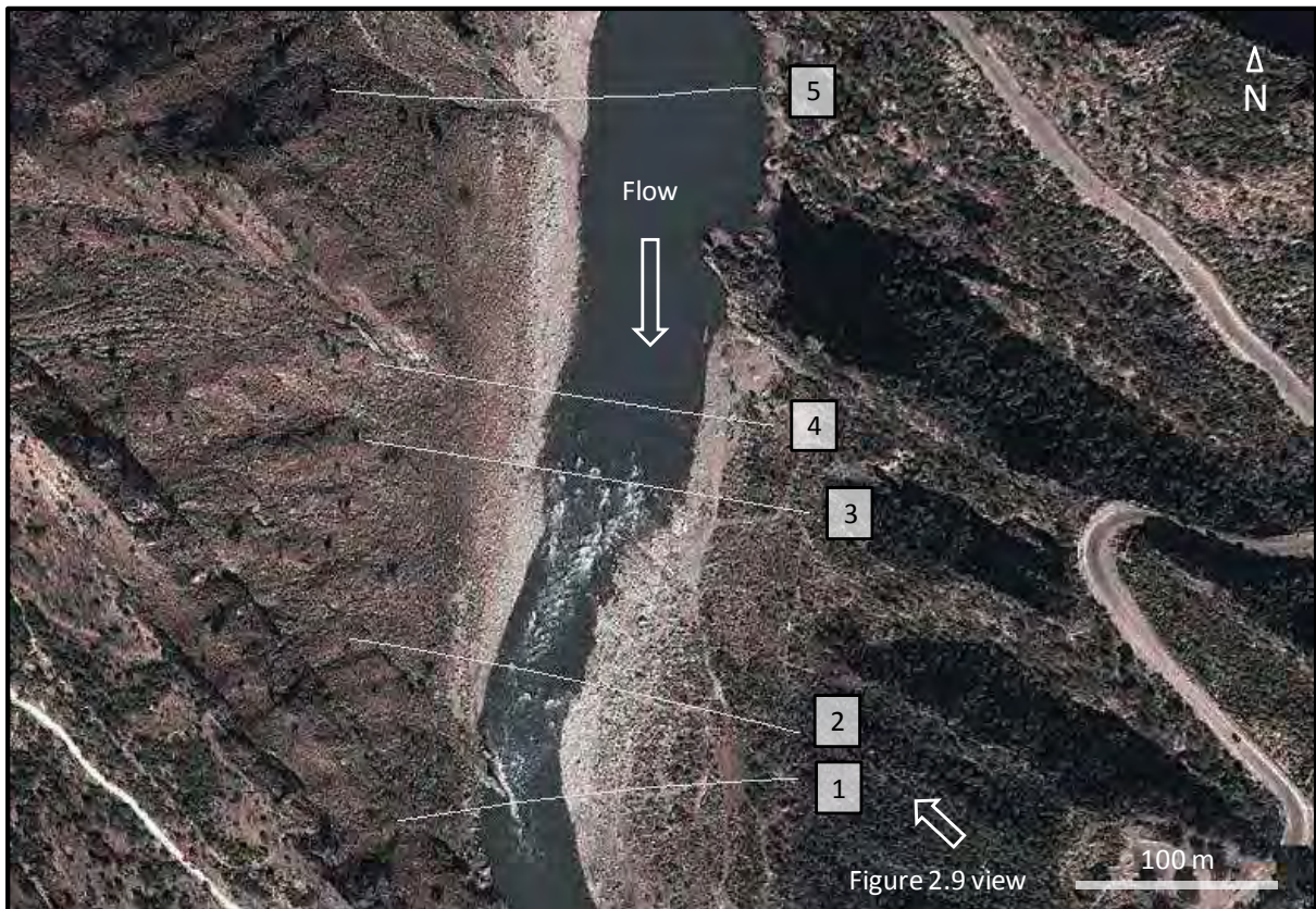
Figure 2.8 The positioning of surveyed cross-sections at EF Site 4 (Billiporian Bridge) using a 9 February 2013 aerial view.
