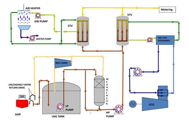
FIGURE-5 PROCESS FLOW CHART – LNG TERMINAL
