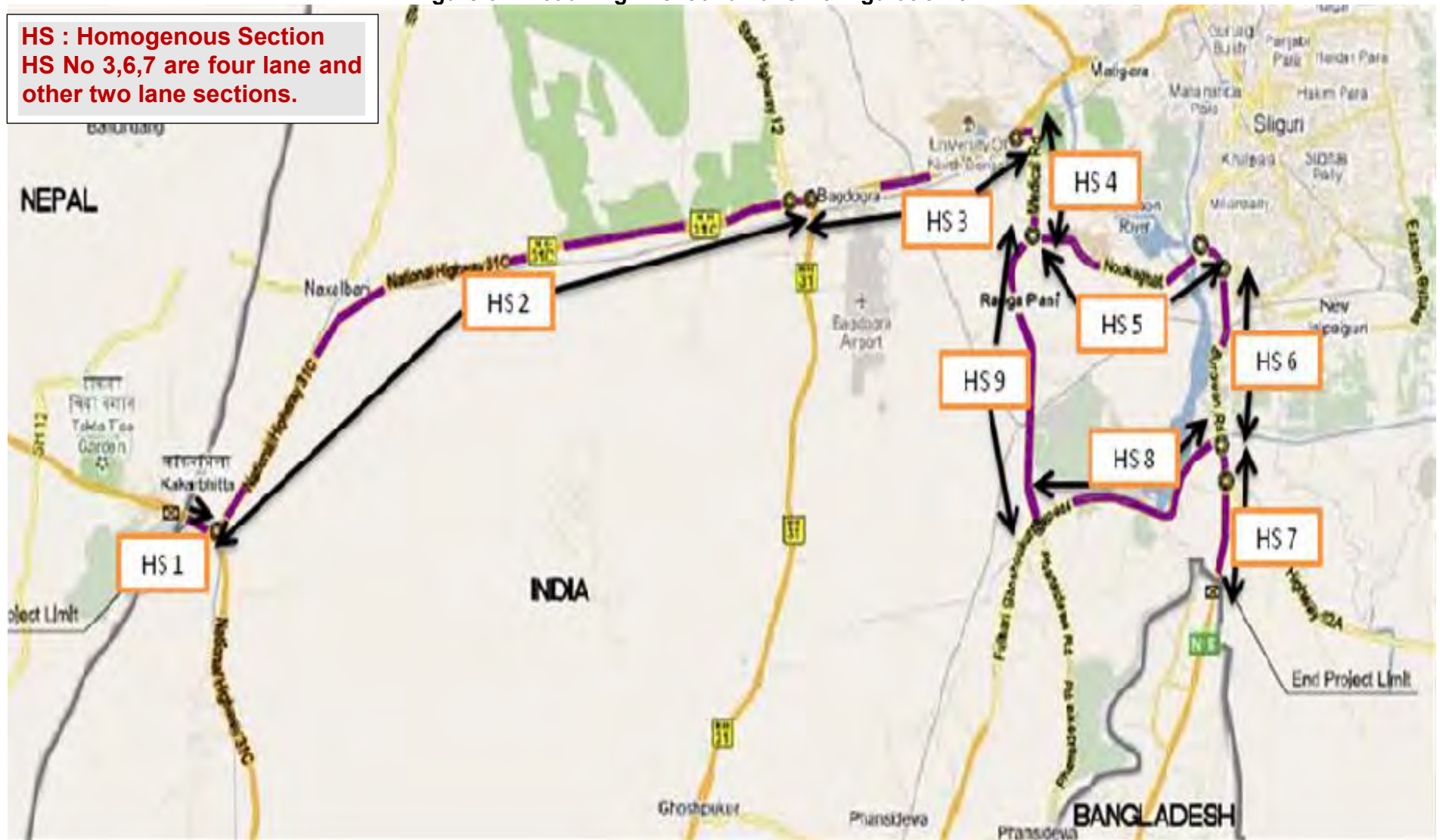
Figure 6. : Road Alignment and Lane Configuration of AH-2
