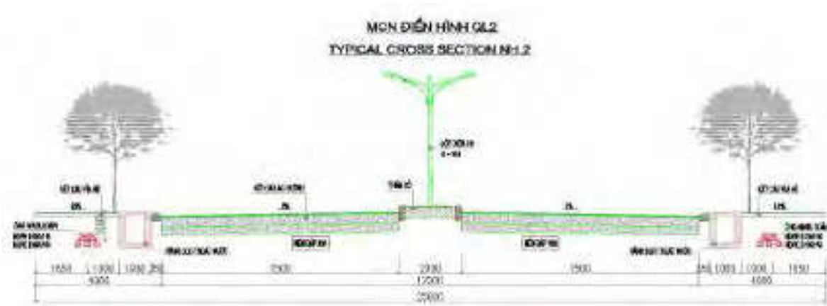
Figure 42. Proposed cross section of upgraded National Road #2
