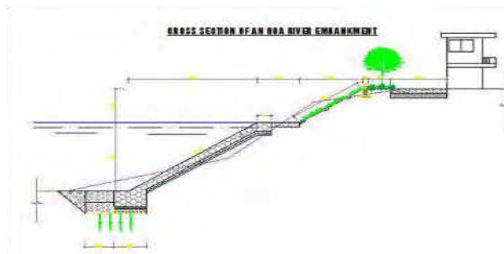
Figure 8. Proposed “green” An Hoa river embankment
