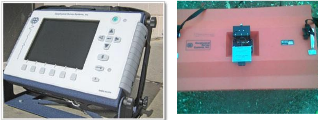
Figure 2: Equipments used for GPR survey
