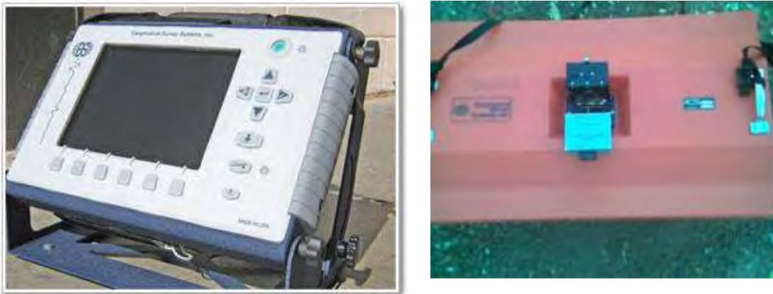
Figure 2: Equipments used for GPR survey
