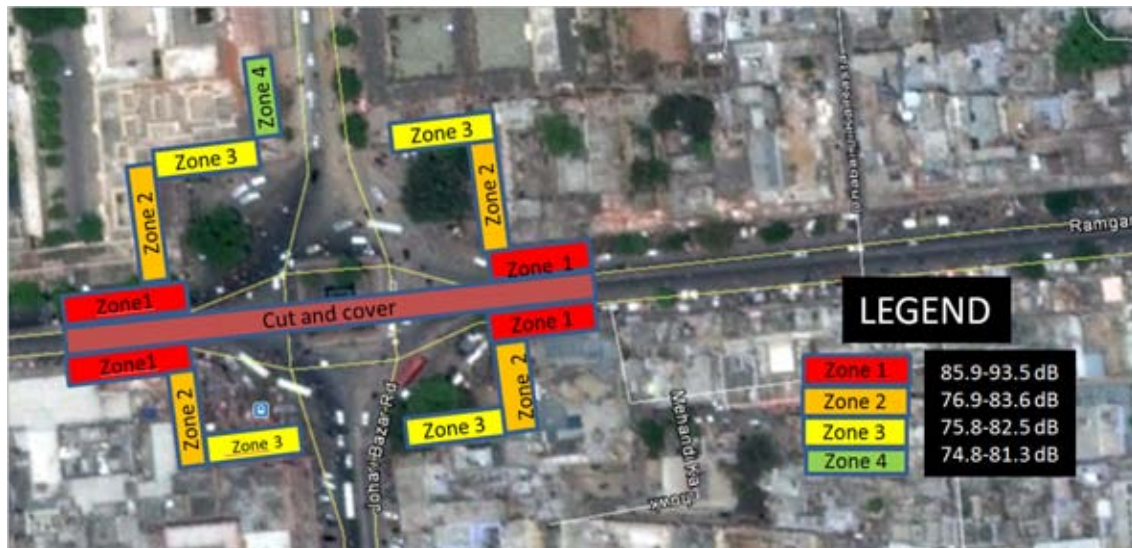
Figure 26: Predicted Noise Level at the Badi Choupar during Cut and Cover Operation
