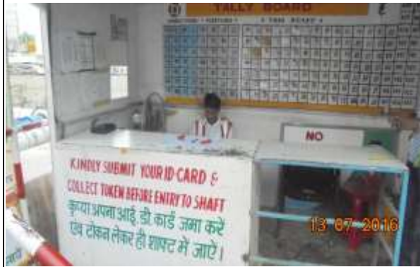
Tally Board system at Chandpole
