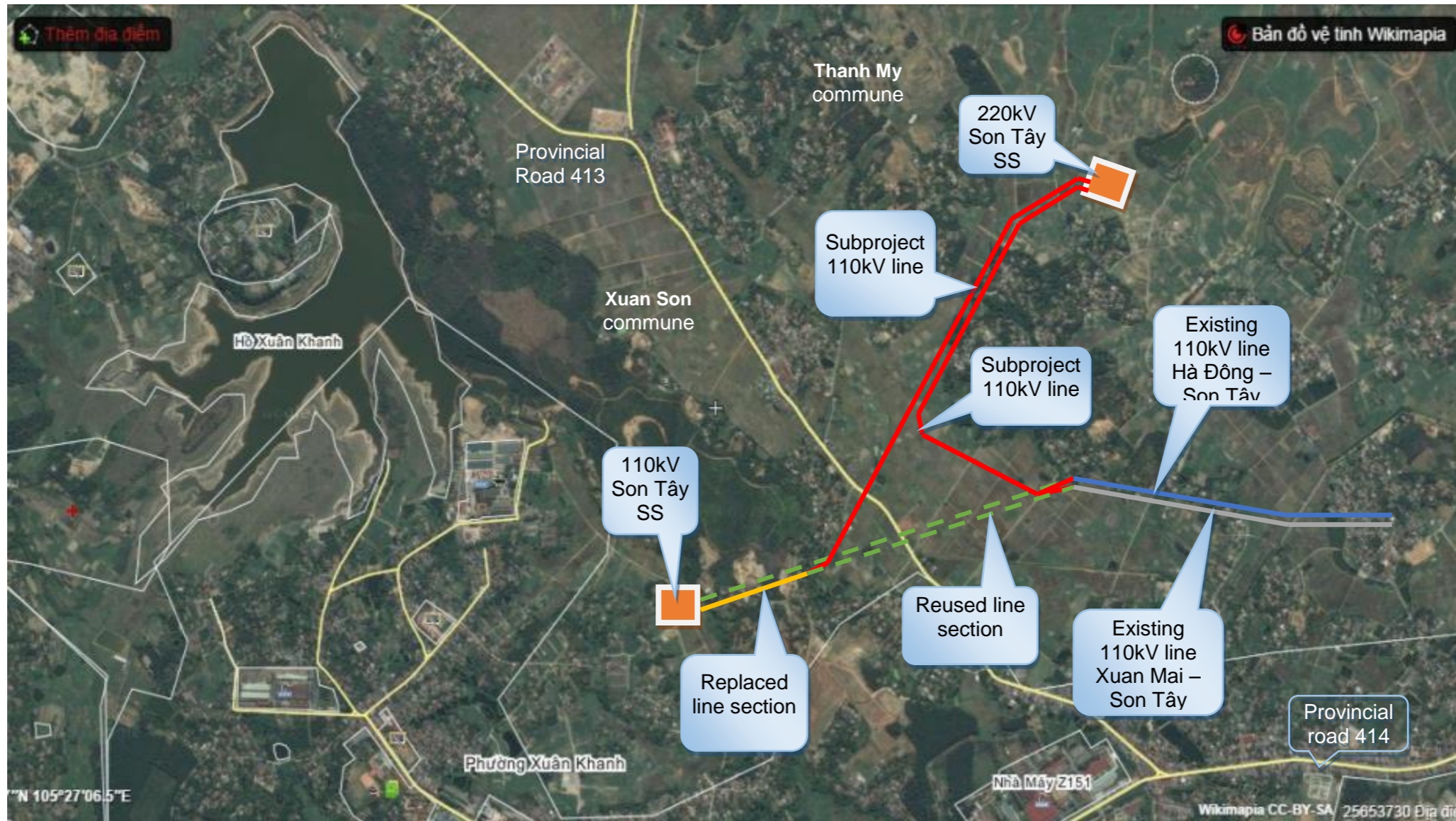
Figure 1 Subproject layout and components
