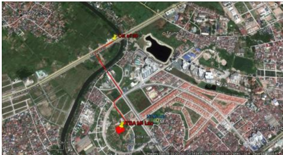
Figure 1. Site of new Mo Lao 220 kV substation and underground cable
