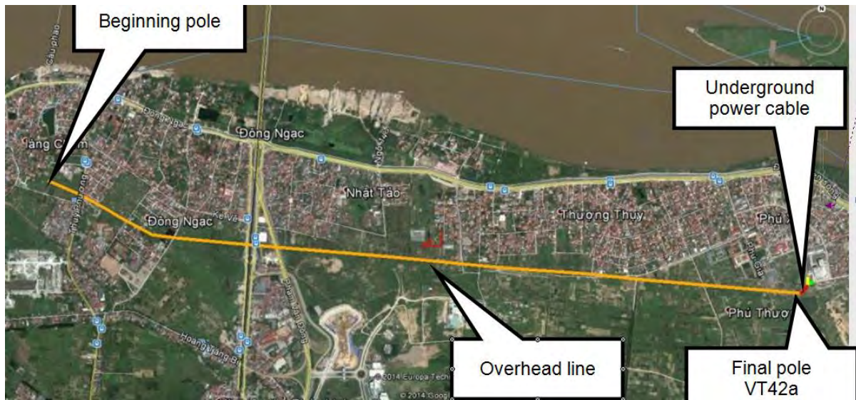
Figure 2: Location of OHL and UGC sections of new transmission line
