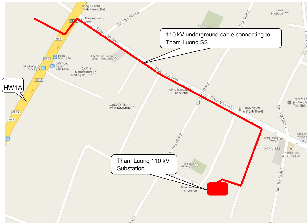
Figure 1. Route of 110 kV Underground Cable connecting to Tham Luong substation and the location of Tham Luong 110 kV substation
