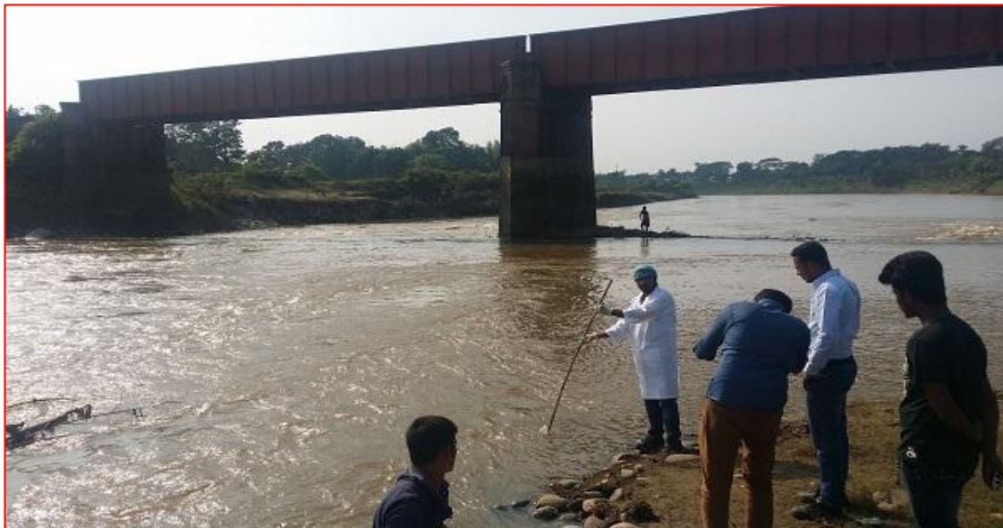
Photo5. Surface water collection near xxx Bridge. Sampling was done according to Engineer's specification
