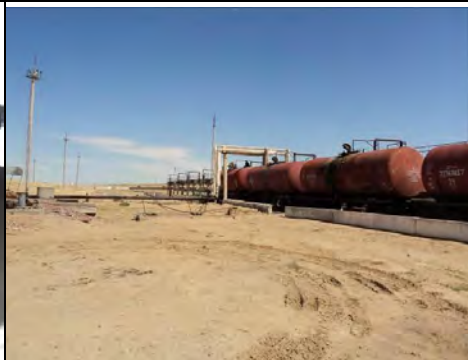
Cisterns on the railway are being filled with residual mazut to be transported to Taskent by train.
