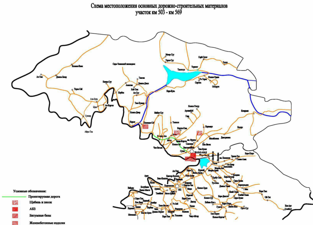
Fig. 7: Borrow Areas along the Road Section Madaniyat–Jalal-Abad
